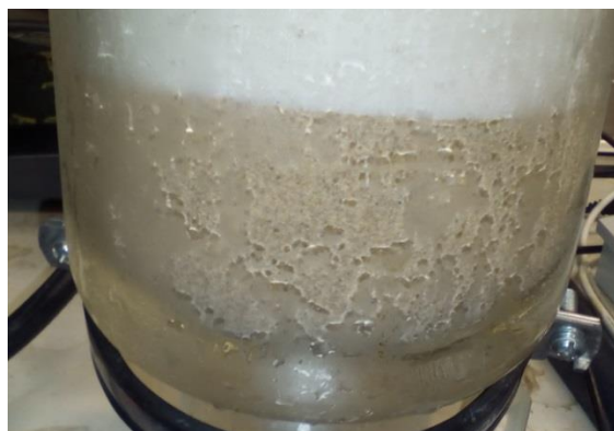
Figure 11 Spontaneous nucleation due to mixing problems in an STR batch reactor experiment
