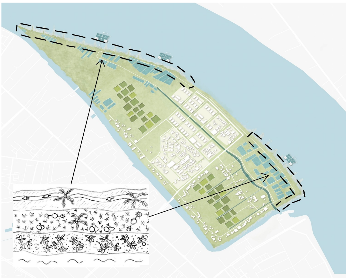
Figure 6.2: A design of Cồn Khương Island in 2075 with the locations for the soft dikes and groynes highlighted (by all authors, 2024). The locations for the soft dikes are based on the risk areas as presented in chapter 12.
