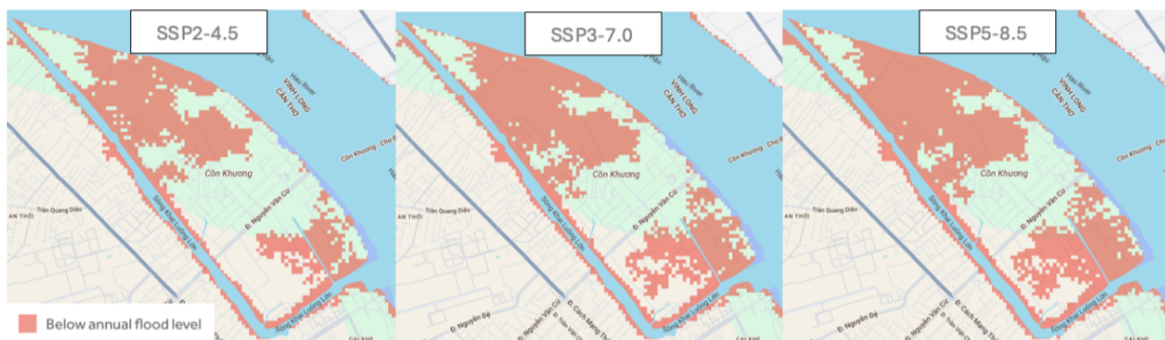
Figure 5.6: Flood scenarios for 2080 in Cồn Khương under the SSP2-4.5, SSP3-7.0, and SSP5-8.5 scenarios, not taking into account subsidence.
