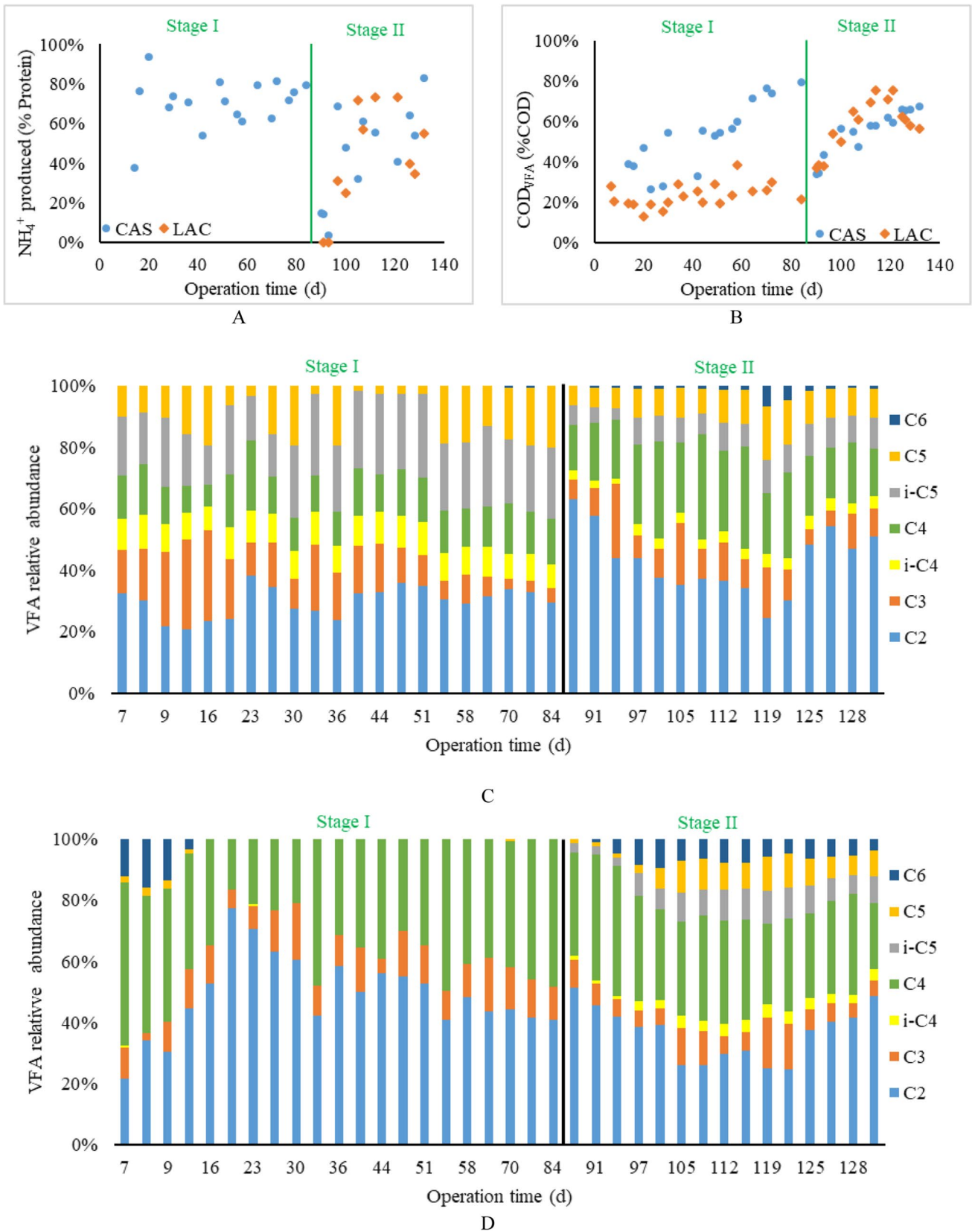
Fig. 3 Deamination (A) and VFA production as % of effluent COD (B) in CAS reactor and LAC reactor during the operational period, VFA relative abundance in the CAS reactor (C), and VFA relative abundance in the LAC reactor (D)
