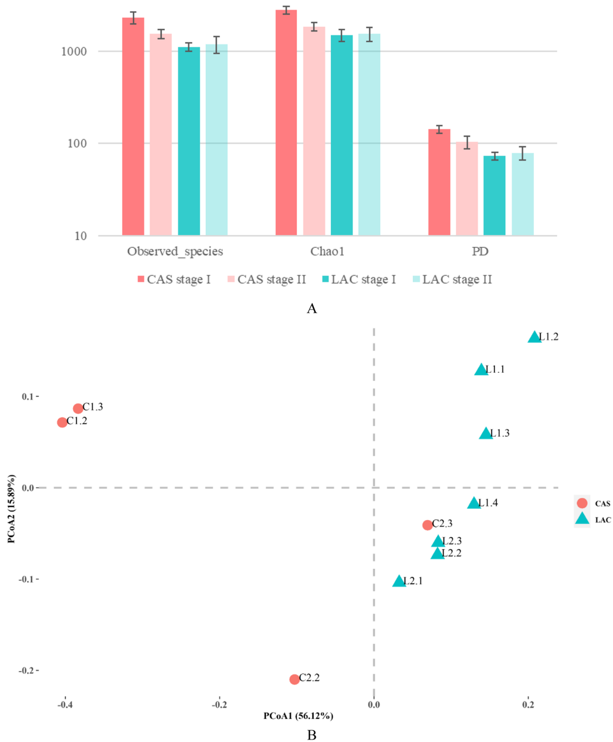
Fig. 6 Alpha diversity of the microbial community in CAS and LAC reactors during stage I and stage II, average values of the observed species, Chao1, and phylogenetic diversity (PD) are presented and the error bars indicate the minimum and maximum values of the samples in each stage (A), Principal coordinates analysis (PCoA) ordination based on the weighted unifracs distance matrix of OTUs comparing all samples taken from CAS and LAC reactors during stage I and stage
