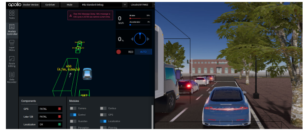
Fig. 8. Screenshot of the SVL-Apollo co-simulation, including PEM. Bounding boxes in \hat{\mathcal{W}} are consistent between Apollo (left) and SVL (right), even undetected objects.
