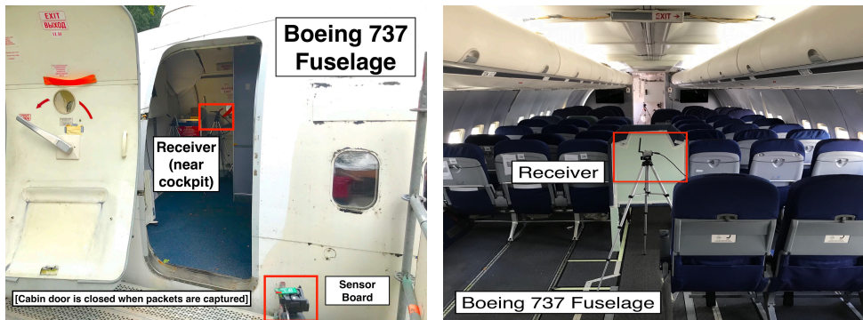
Figure 6.4: Sensor wireless signal transmission experimental setup inside a Boeing 737 fuselage.
