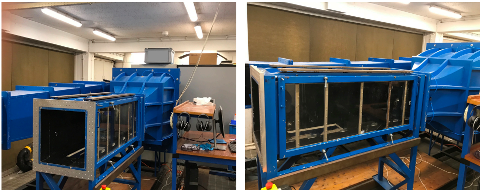
Figure 3.1: Low speed wind tunnel used for controlled experimentation.
