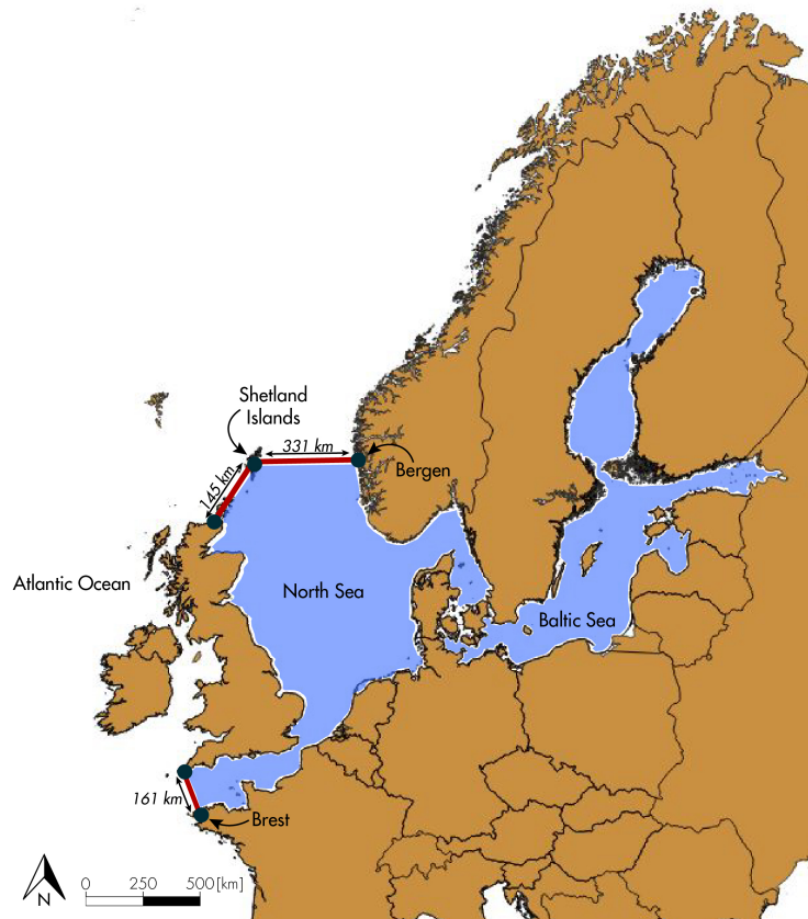
Figure 1.1: The location of the NEED (in red) and the enclosed basin consisting of the North Sea and the Baltic Sea (in blue), as proposed by Groeskamp & Kjellsson (2020).
