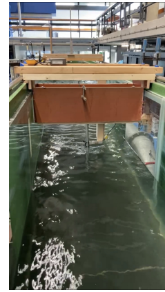
Figure 3.2: Two structures to make the cylinder rigidly fixed. Figure (A) was used for all cylinders except for the smooth cylinder with a diameter of 2.5 cm.
