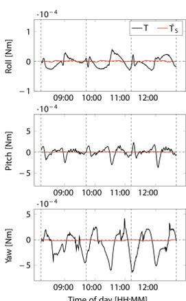
Solar radiation pressure causes the second to largest non-gravitational disturbance force in LEO, but the resulting torques are generally small. Due to the symmetric nature of GOCE, these effects are reduced even more. A similar model is used as for aerodynamic torques, with **force and moment coefficients** from a Monte-Carlo simulation in ANGARA\* and the **sunlight vector** derived from the spacecraft attitude and the sun position from the Spice toolbox.
