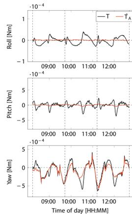
Improving the aerodynamic model is the main goal of this research, but for now a default model is used. The **force and moment coefficients** are obtained from a Monte-Carlo simulation in ANGARA\*, as a function of aerodynamic angles and speed ratio. **Temperatures and particle densities** from NRLMSISE-00 are used to interpolate on these coefficients, while **GOCE density and cross-wind data** are used for the actual torque calculation.
