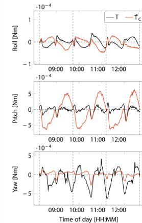
Attitude control is realized by three magnetic torquers aligned with the three body axes of the satellite. The **current** through the torquers is available from the housekeeping data. These currents are converted to **dipoles** using an adaptive cubic polynomial model. Together with the calibrated **magnetometer field measurements** the control torque is obtained.
