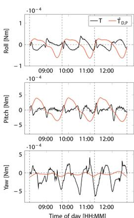
Dipole models are only available for the spacecraft bus, not for the payload and instruments. Therefore a **constant hard magnetic** and a **constant soft magnetic** dipole are fitted to the residual torque over four orbits on December 1<sup>st</sup>, 2009. On this day the solar activity was low, leading to a small aerodynamic contribution.
