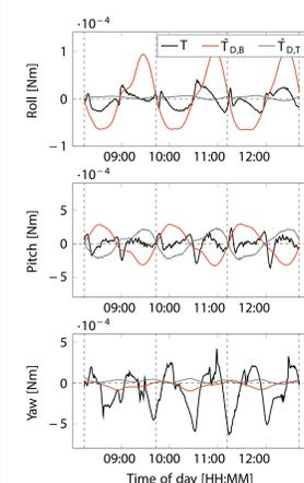
The spacecraft bus contains many elements apart from the torquers that generate a magnetic dipole. These dipoles again cause a magnetic torque depending on the **Earth magnetic field** direction. Based on the results of a hook test performed on GOCE during development, a **hard magnetic dipole**, as well as several **soft-magnetic dipoles** are modeled. On top of that the magnet of the **ion thruster** causes a significant dipole (shown separately in the plot).
