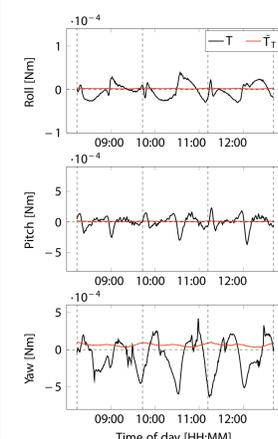
The ion thruster is aligned such that the thrust vector acts exactly between the beginning- and end-of-life centers of mass. This means that most of the time, the **thrust** will have a slight offset from the **center of mass**, causing a torque. As the center of mass only shifts slowly, the torque trend is equal to that of the thrust force.
