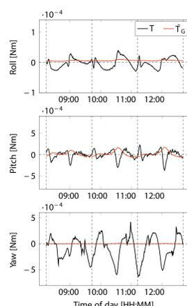
Gravity gradient torque is generally considered to be one of the major attitude disturbances to satellites in low orbits. Assuming a simple model, yet incorporating the **gravity vector** from EGM2008, this torque can be calculated. The **inertia tensor** is linearly interpolated between the beginning- and end-of-life values.
