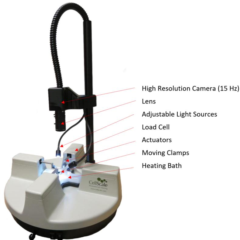
**Figure 2.6:** Commercial uniaxial tensile tester with the components referred to [CellScale Biomaterial Testing, Waterloo, Canada]
