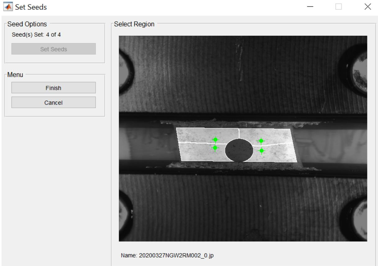
**Figure C.7:** The selected seeding points, which equal to number of cores selected under RG-DIC Parameters (4). It is important that the seeds are placed so that the regions are subdivided somewhat symmetrically as seen in this figure
