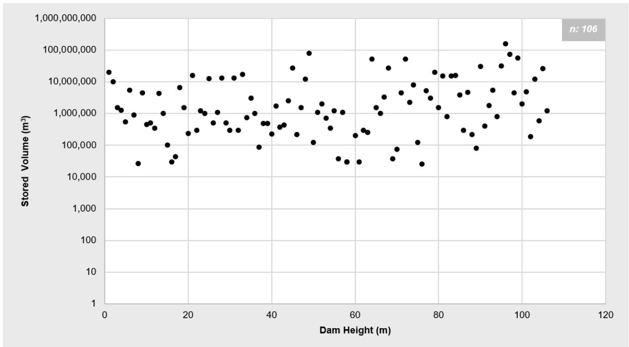
Figure A.14: Dam Height versus Stored Volume
