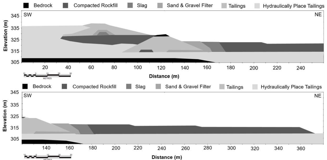
Figure C.13: Sketch of Cross Section 2022
