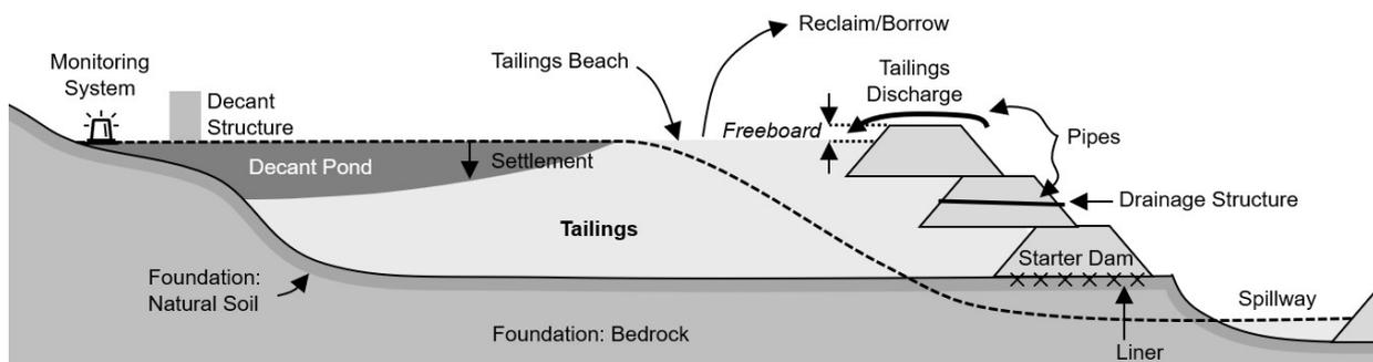
**Figure 2.5:** Main Components of a Tailings Dam
