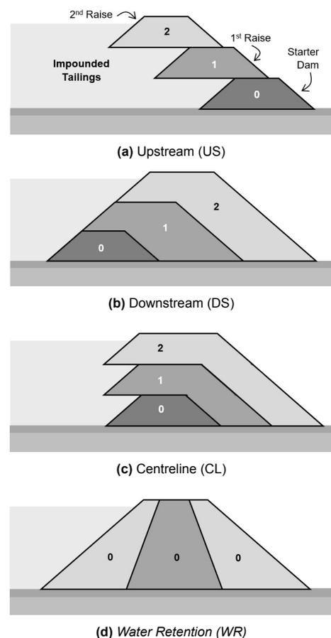
**Figure 2.4:** Common Dam Construction Methods
