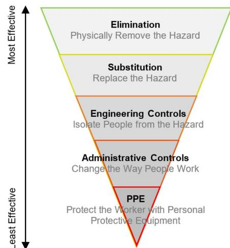
**Figure 3.2:** Hierarchy of Controls
