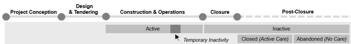
**Figure 2.2:** Schematic Overview of General Lifecycle of a Tailings Storage Facility (TSF)
