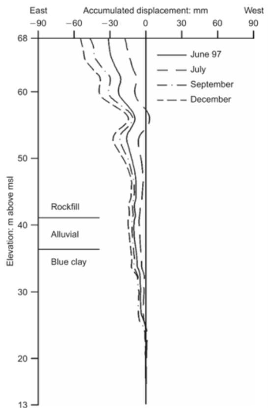
**Figure C.9:** Inclinator Readings (Alonso & Gens, 2006a)
