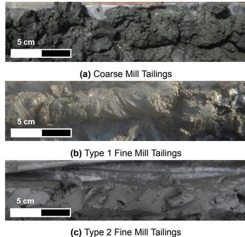
Figure C.15: Close-Up Picture Mill Tailings
