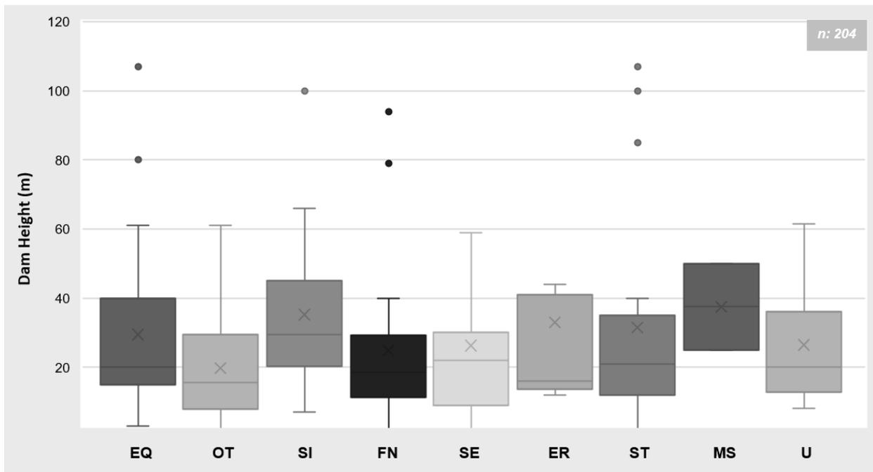
**Figure A.11: Dam Height by Failure Category**
