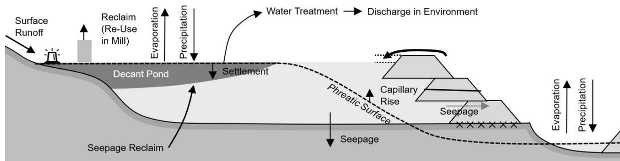
Figure 2.6: Water Balance of a Tailings Dam
