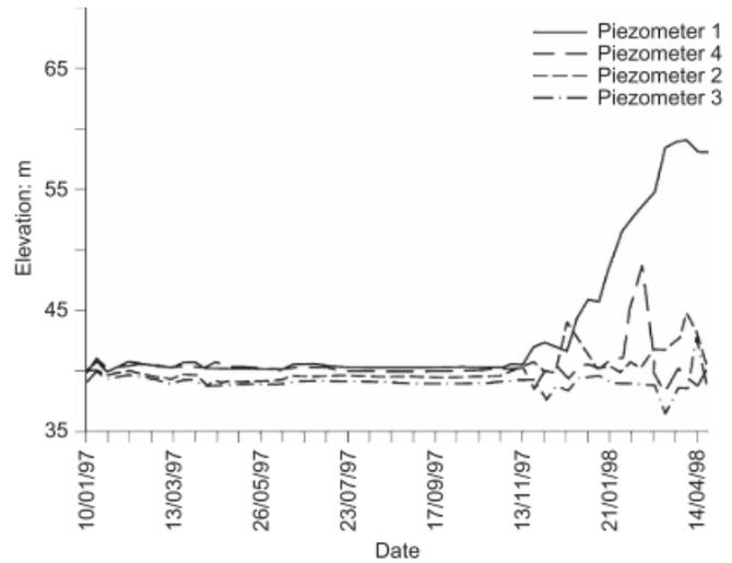
Figure C.10: Piezometric Readings (Alonso & Gens, 2006a)
