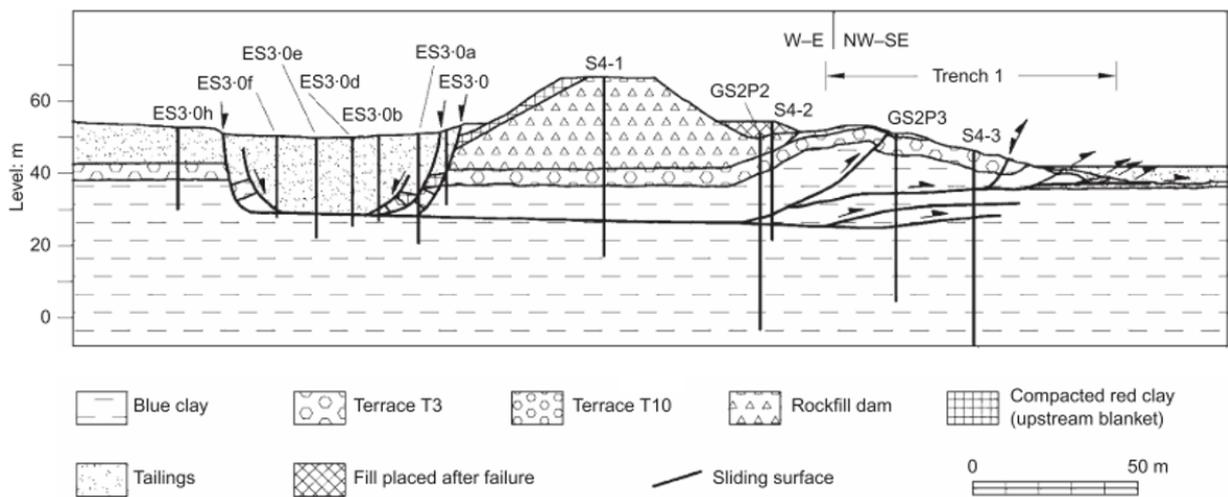
Figure C.2: Cross Section of Slide showing Failure Surfaces (Alonso & Gens, 2006a)
