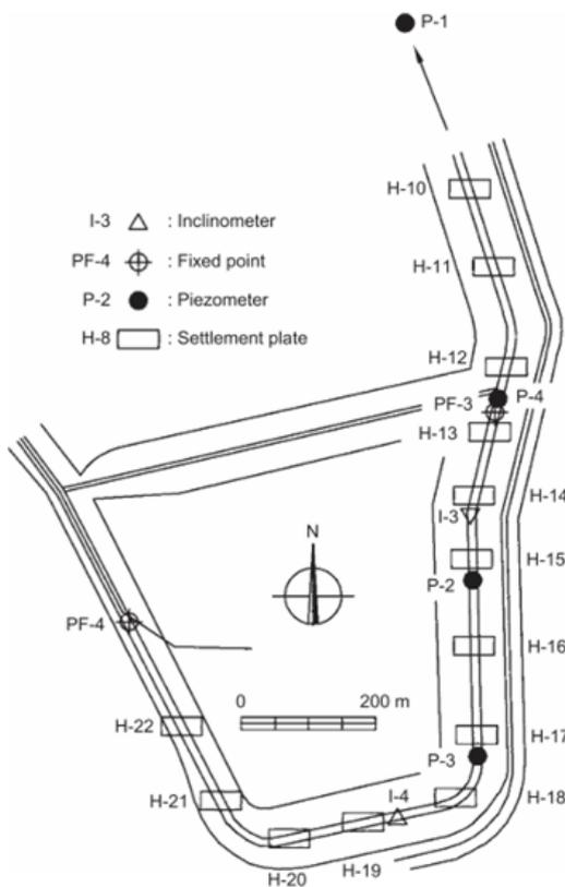
**Figure C.8:** Overview of Position of Monitoring Instruments (Alonso & Gens, 2006a)
