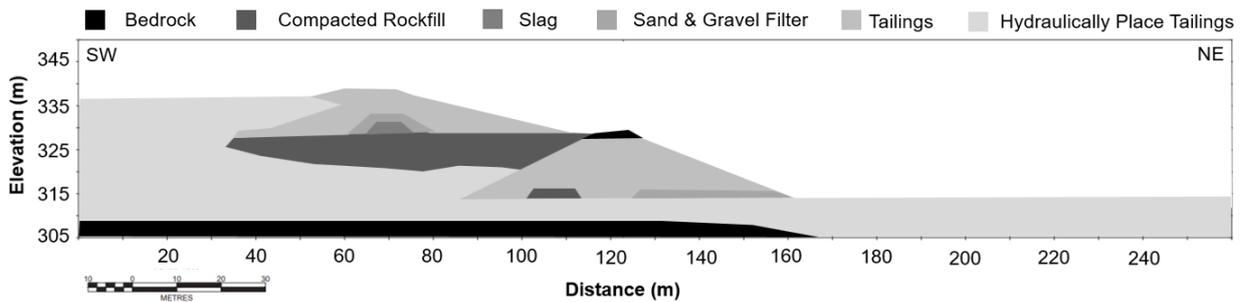
Figure C.12: Sketch of Cross Section 2017
