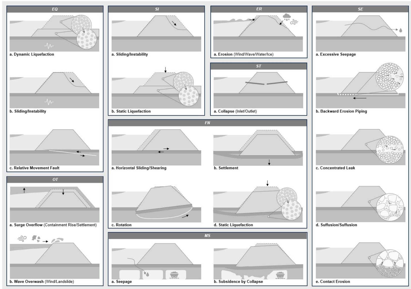
Figure 2.7: Schematic Overview of Different Failure Categories
