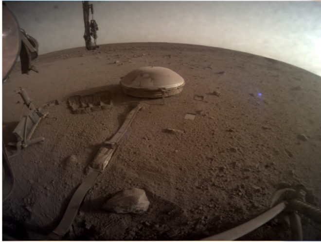
FIG. 1 Instrument context camera view of the wind and thermal shield (WTS) covering the SEIS seismometer in the center and the HP3 device on the left-hand side. The foot consists of a disc with 60-mm diameter and a 20-mm-long conic spike (10-mm diameter at its base) in its center (Image Credit: NASA/JPL-Caltech: _mars.nasa.gov/insight-raw-images_surface_sol_1436_icc_CO00M1436_724026383EDR_F0000_0200M_ ).
