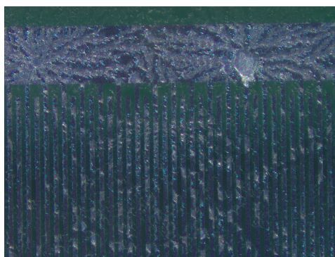
Figure 9.23: Microscope image of PCB 9 after 16 hours pass since the HMDA step (during the day long dry period) showing some crystallised material (expected to be HMDA) on the IDT.
