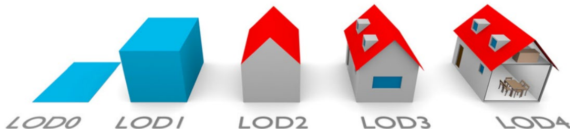
Figure 8: The five LODs of CityGML 2.0 on the example of a Building. Taken from Biljecki et al., 2016.
