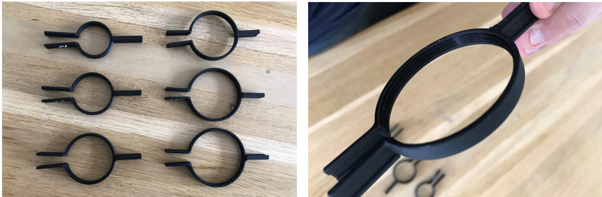
(a) 3D printed hydrostat clamps in various diameters.
