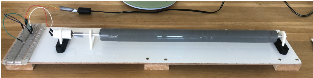
(c) Final cured silicone sleeve on the PVC pipe.
