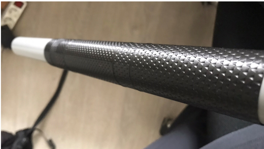
Figure H.44: PVC pipe with several textured molds: debossed triangle shape, debossed dotted shape, and embossed triangle shape.
