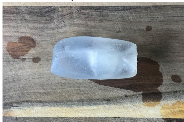
(f) Step 6: Finalized hydrostat
