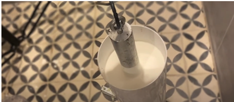
Figure C.18: Latex dipping method (5): A heated rod is dipped in liquid latex. The latex solidifies against the rod and is pulled out of the bath at a constant speed to ensure a smooth finish.
