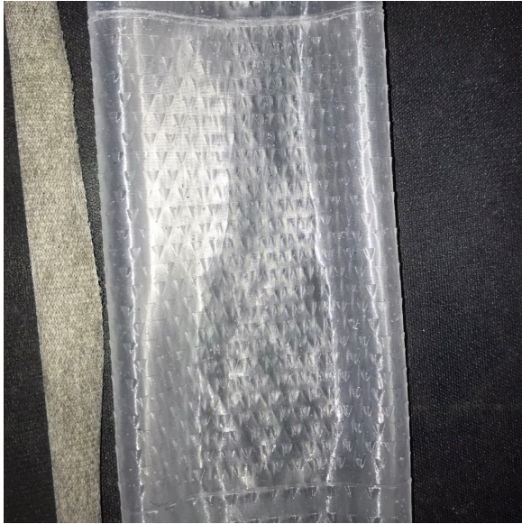
(a) Triangle pattern embossed on the sleeve.
