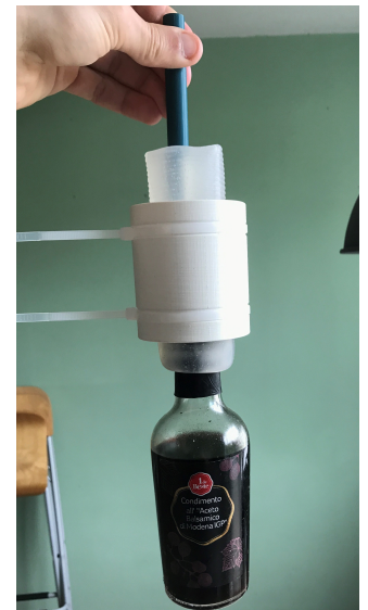
(b) Hydrostat gripper with hand-held device holding a bottle.
