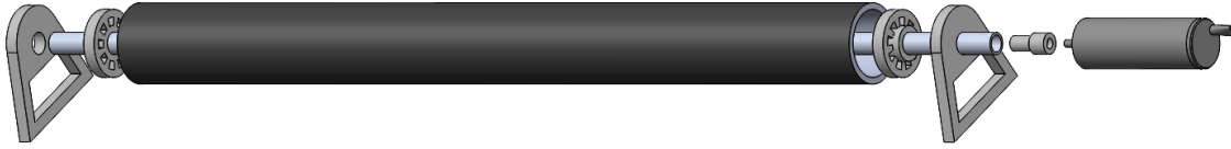
(a) Exploded view of the manufacturing rig consisting of a PVC pipe, an aluminum rod, 3D-printed mounting brackets and inserts, and a 12V-DC motor.
