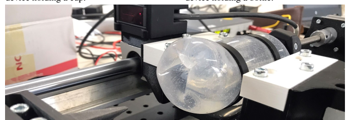
(c) Hydrostat gripper in the experimental test.
