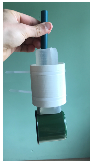
(a) Hydrostat gripper with hand-held device holding a cup.
