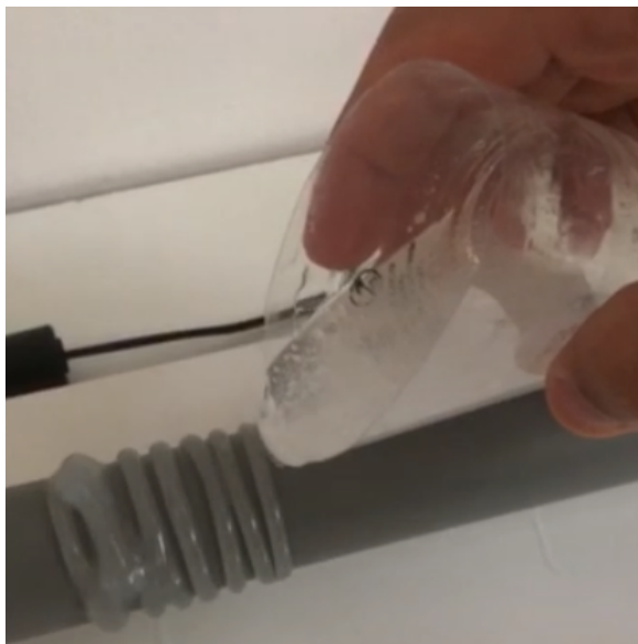
(a) Pouring liquid silicone onto the PVC pipe at a constant speed.
