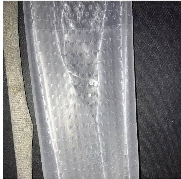
(b) Triangle pattern debossed in the sleeve.
