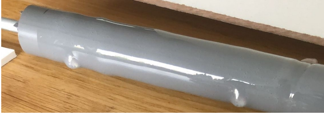
Figure C.21: Silicone droplets forming on the sleeve due to excessive silicone use.
