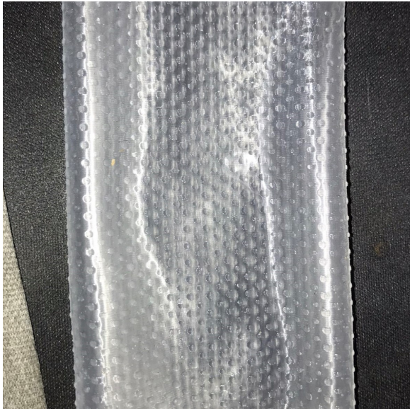
(c) Dotted pattern embossed on the sleeve.
