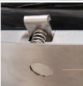
Button to open frame, letting bottles and cans out
