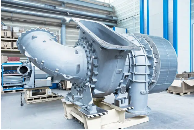
Figure 3.2: Real-scale turbocharger for marine ICE applications. The turbocharger is composed by the compressor and the turbine coupled to the same shaft. As a result, it serves as the interconnection between \Sigma^{(3)} and \Sigma^{(4)} (Image credits: ABB)
