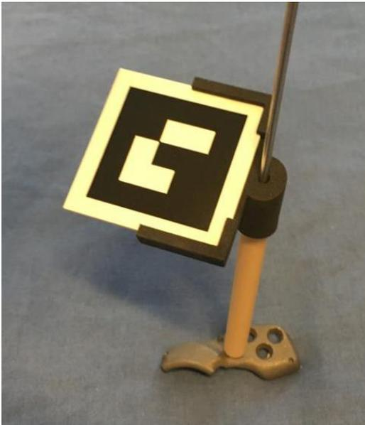
Figure 17: Navigation tool including the fiducial attached to the implant via an 8.0 cm drill guide (scenario 1). The drill is inserted in the drill guide.
