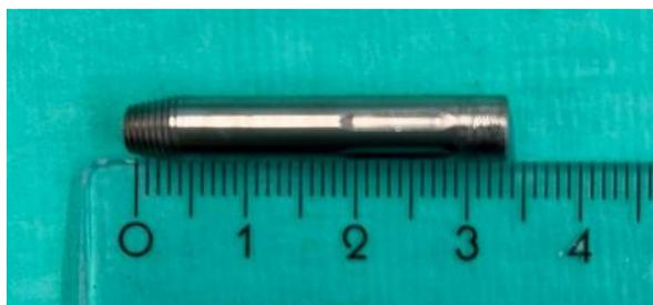
Figure 16: Metallic drill guide of approximately 3.5 cm.
