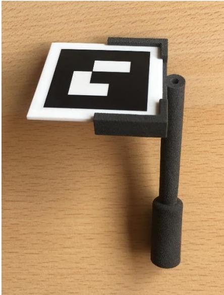
Figure 19: Navigation tool to be used in combination with the 3.5 cm drill guide. The lower part contains the part that slides over the metallic drill guide.
