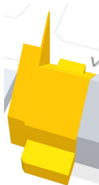
Figure 9. An example of a model with a “screen”. This model has an RMS of 0.04 m, and a maximum model-to-point distance of 6.1 m.
