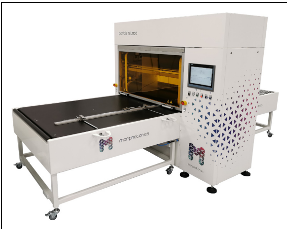
Figure 4. Morphotonics Portis NIL1100 roll-to-plate nanoimprint equipment. 41
