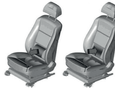
Figure 2.7. "roll function" in the lumbar support by Franz et al. (2010).
