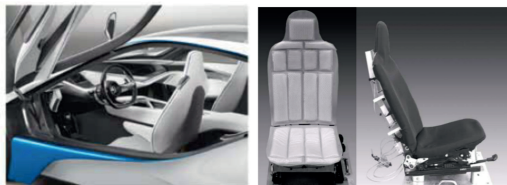
Figure 2.28. . Prototype of thin profile seat by Franz et al. (2011)
