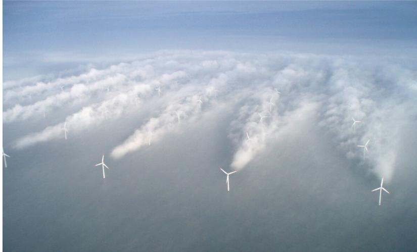
**Figure 2-4:** Picture of wakes in an offshore wind farm [3].
