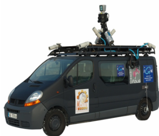
Figure 9 The mobile mapping system of IGN
