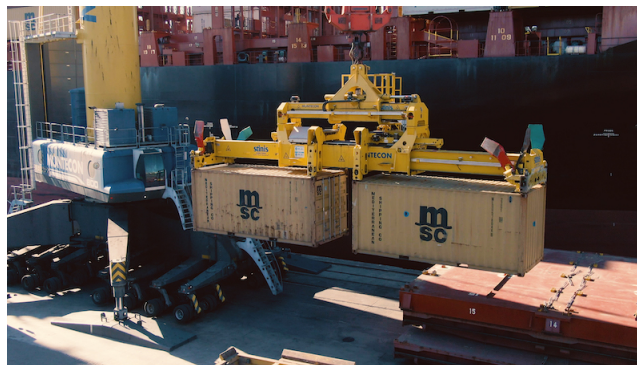
Figure 3.8: Twin Spreader Technology [60]
