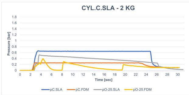
Fig. 17. Pressure development in cylinder C.SLA with a 2 kg weight attached for 20 seconds
