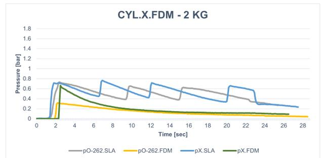
Fig. 23. Pressure development in cylinder X.FDM with a 2 kg weight attached for 20 seconds
