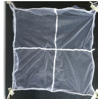
Test Setup 2 Hemp Rope with 1x1 Ribs
