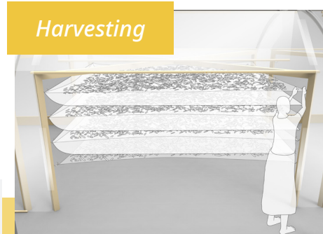
21. Unhook the short side of the top net and the guiding sheet beneath it
