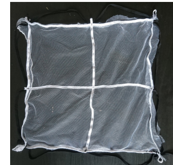
Test Setup 6 Elastic bands with 1x1 Ribs and support ropes on the sides
