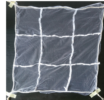
Test Setup 3 Hemp Rope with 2x2 Ribs
