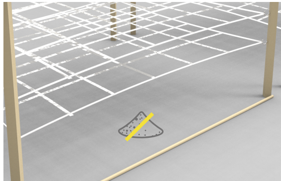
The lifted drying nets keep the dagaa away from sand contamination.
