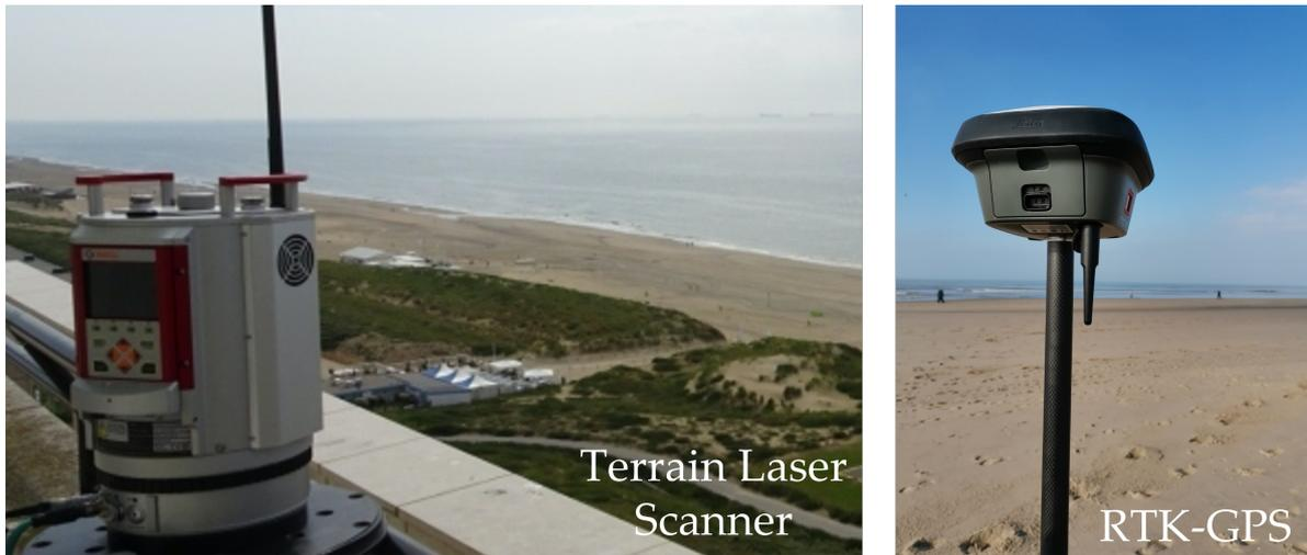
**Figure 3.5:** Validation devices: TLS RiegIVZ-2000 (left) and RTK-GPS Leica GS18i (right).
