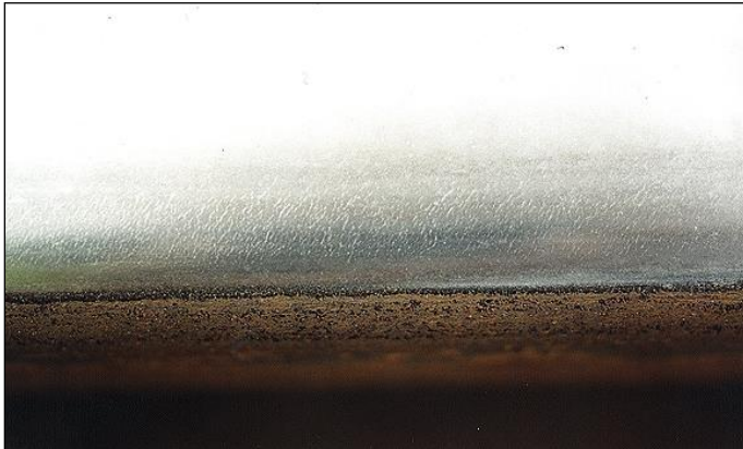
Fig. 3. Fine network of superficial cracks (craquelure) on the premium rail grade (site B). Direction of traffic is to the left, depicted rail length is about 0.1 m.
