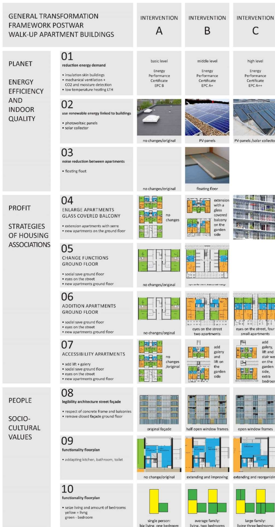
Figure 8. Design variations of the VAM walk-up apartment building are categorized in a choice matrix, GTF, for option appraisal. The most common postwar floorplan type E3 designed by the architect E.F. Groosman is used. Graphic by Leo Oorschot.
