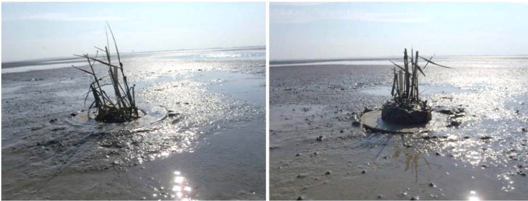
Fig. 2. Visual presentation of the concrete-rings-method, used to mimic a stable non-eroding mudflat with a constant height (i.e., \delta z_{TF} = 0 ) adjacent to marsh sediment (i.e., the marsh core). A height difference between the mudflat and marsh core ( \Delta Z ) can be created artificially by raising the core in the concrete ring, and mimics in a simplified way the height difference as will be obtained due to sediment dynamics on the tidal flat ( \delta z_{TF} ) adjacent to a marsh with more stable sediment.
