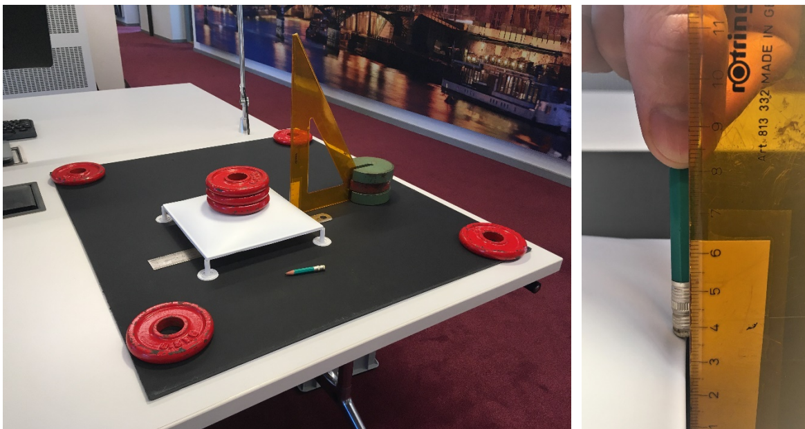
Figure 15 Physical model (left) and manually applied vertical load at the edge (right)
