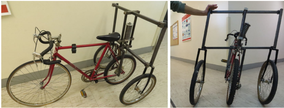
Fig. 12 A 'bricycle': a vehicle which can transition between a bicycle and a tricycle [64]
