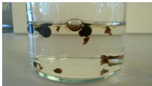
Figure 2-10: Aggregates of Ca-ALE, after ALE was dropwise added to a CaCl 2 -containing solution.
