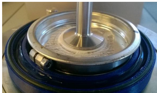
Figure 5-2: A particle containing Ca-alginate gel in the rheometer, with the bottom part of the liquid trap.
