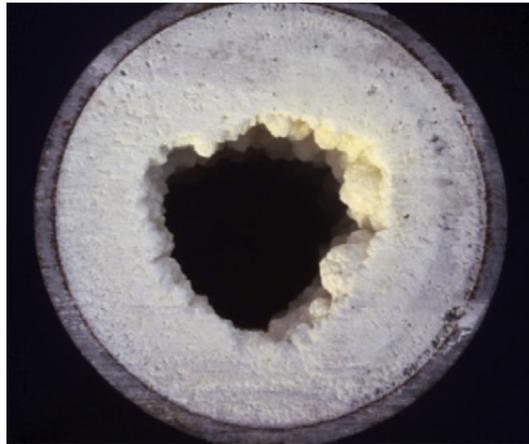
Figure 1.1: Calcite scaling in a well after three weeks [1]
