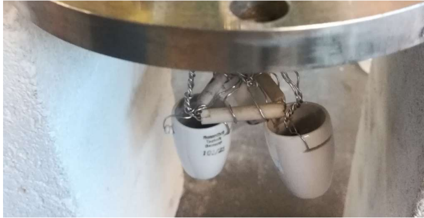
Figure 23. The three ceramic crucibles containing the sinter material (top= 2 cm, bottom = 1 cm, height= 3.5cm).
