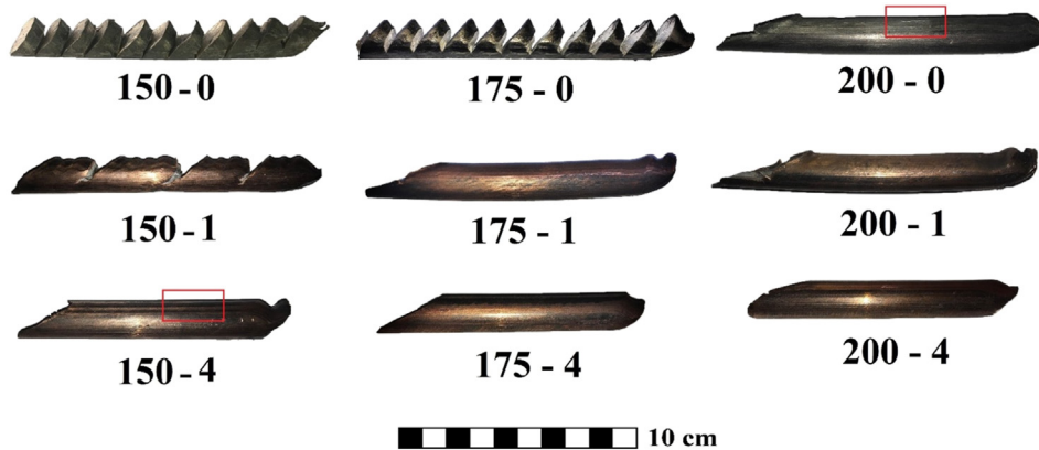
Fig. 6 – Samples with CTC of different thicknesses, deformed at different temperatures.
