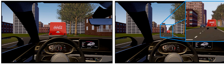
Fig. 1. Participants' view of the task in the driving simulator. As the vehicle driven by a participant approached an intersection, the truck in the participants' lane started moving away, revealing the oncoming car. The participants had to decide whether to go (accept the gap and turn left before the oncoming car), or stay (reject the gap and turn left after the oncoming car passes the intersection). Video recordings of example trials are available in online supplementary information at https://osf.io/5hu7e/ .
