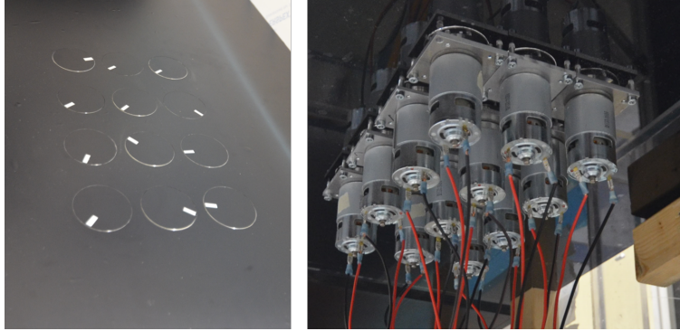
Figure 7.2: Picture of the disc array as viewed from the top and bottom, the white tape on the discs was used to measure the angular velocities using a tachometer.
