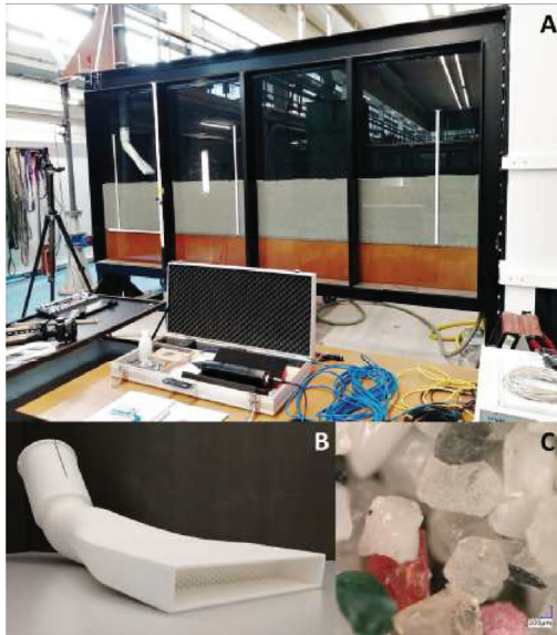
Figure 2: Experimental setup: (a), the 2D and 3D-printed water jet (b), and sediment (c).
