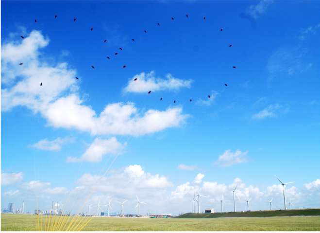
Fig. 12. Composite photo of the 14 m 2 kite flying a figure of eight manoeuvre ( \Delta t = 1s ) on 23 June 2012 at the Maasvlakte 2 of Rotterdam Harbour [24].
