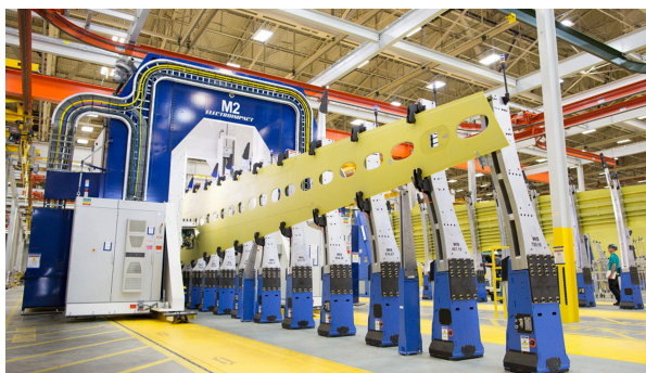
Figure 12.1: Robotic Panel Assembly Line (PAL) used for the wing's assembly 3 .
