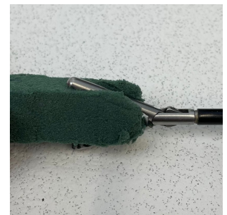
Fig. 23. The forceps of the laparoscopic instrument grasps the Floral foam object.
