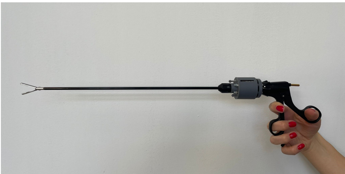
Fig. 25. Prototype of the force limiting mechanism in a laparoscopic instrument.
