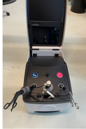
Fig. 18. The boxtrainer with two laparoscopic instruments. The non-dominant hand held the instrument with or without the force limiting mechanism. The dominant hand held the instrument without the force limiting mechanism.
