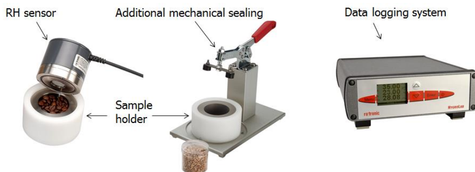
Figure 3. Set-up for the RH measurement.
