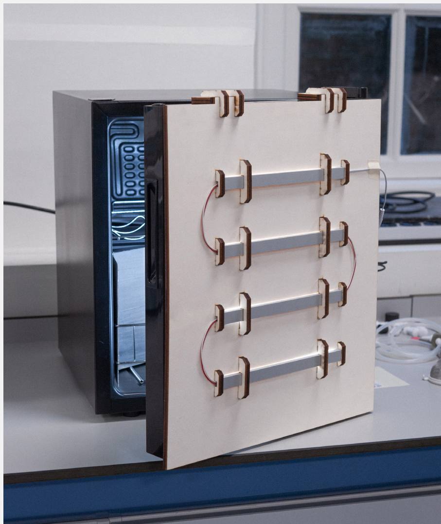
IMAGES [37] OUTSIDE GROWING SETUP LIGHT PANEL WITH ALUMINIUM HOUSING
