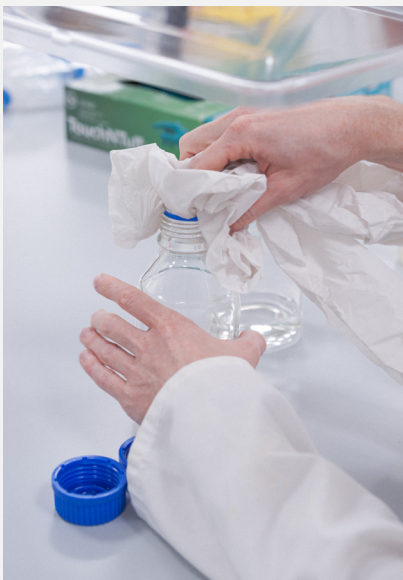
IMAGES [38-39] STERILISATION OF THE CONTAINERS WITH THE USE OF ETHANOL
