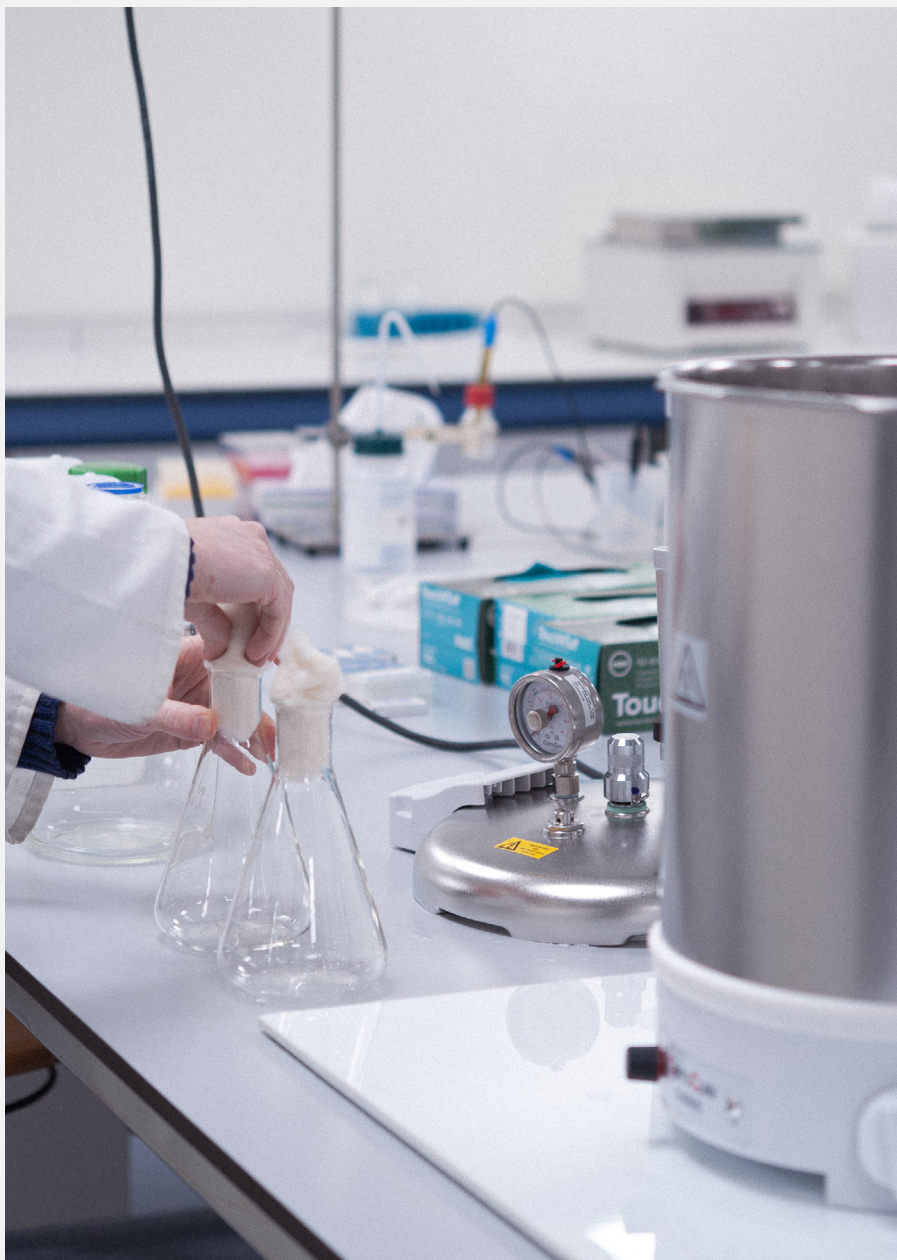
IMAGE [41] STERILISATION PROCESS PREPARING ERLLENMEYER FOR AUTOCLAVE
