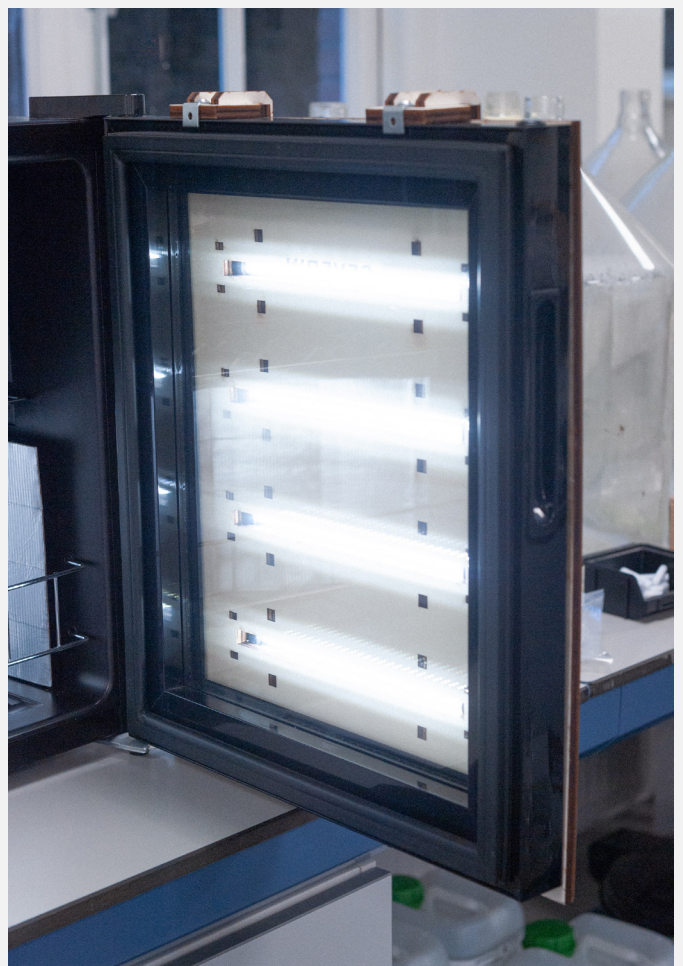
IMAGES [37] OUTSIDE GROWING SETUP LIGHT PANEL WITH ALUMINIUM HOUSING
