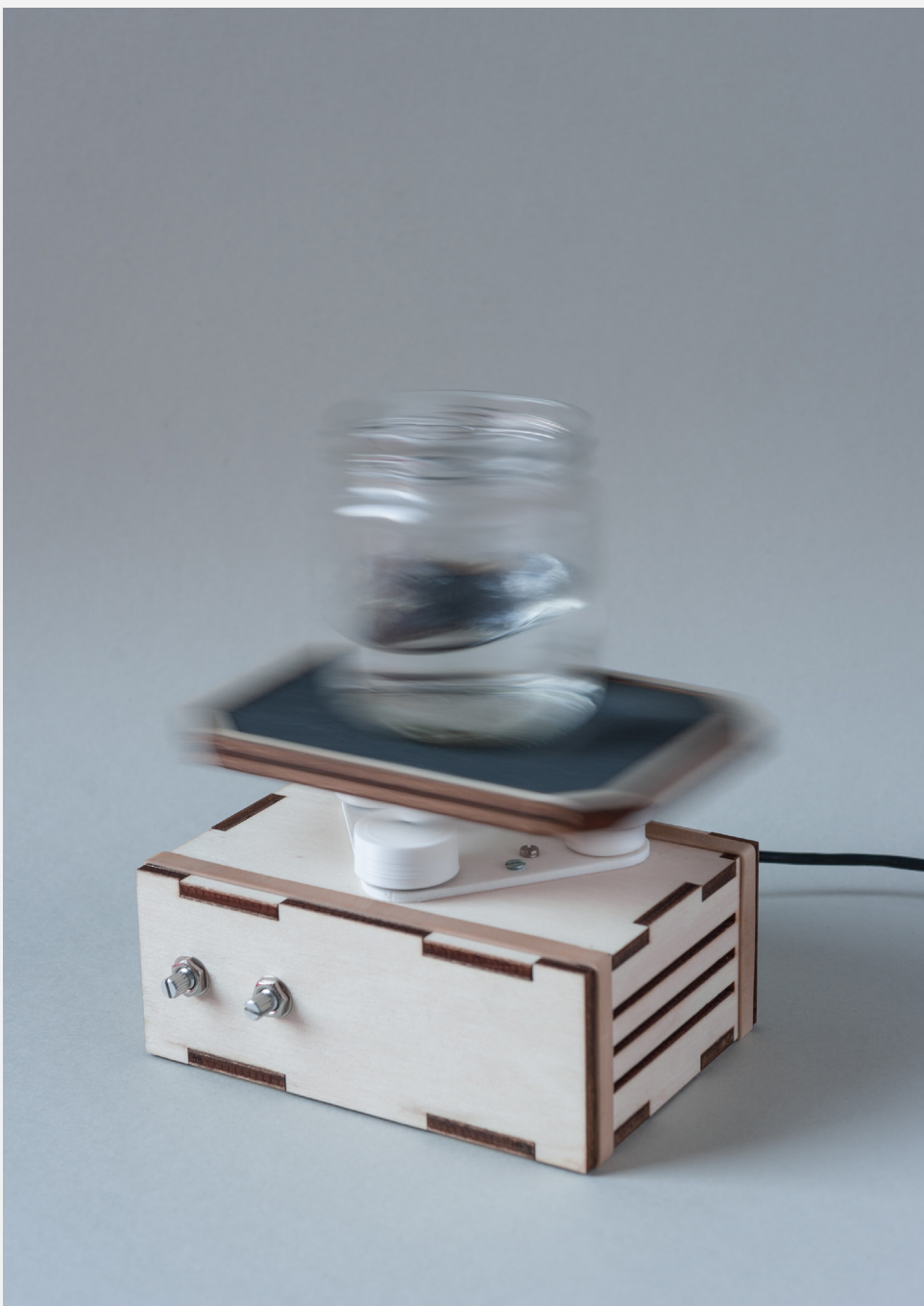
IMAGES [52] OVERVIEW OF ORBITAL SHAKER SILICON MAT TOP
