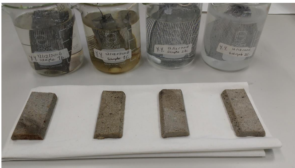
Figure 20: CEM-III Foam concrete samples cut in a rectangular shape and exposed to sulphate and chloride solutions
