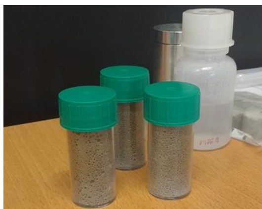
Figure 18: CEM III/B 42.5N LH/SR + Foaming agent, foam concrete used for Neutron Tomography studies
