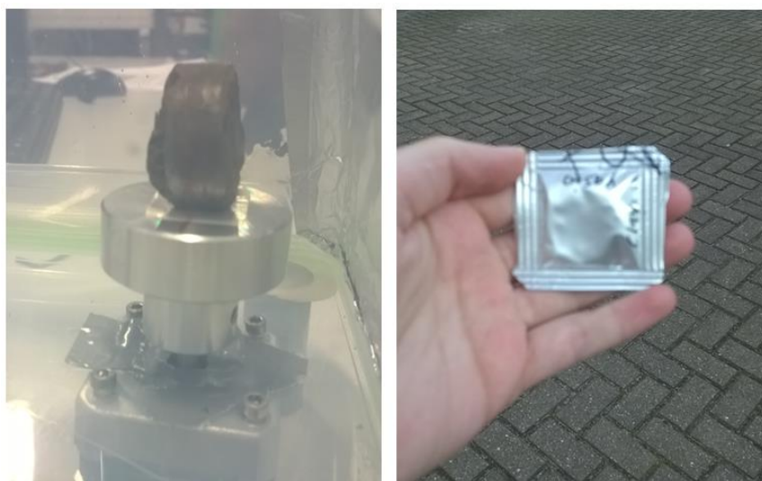
Figure 17: Boom clay on a rotor stage for CT (left) | Boom clay in a metal-foil packet to avoid oxidation (right)
