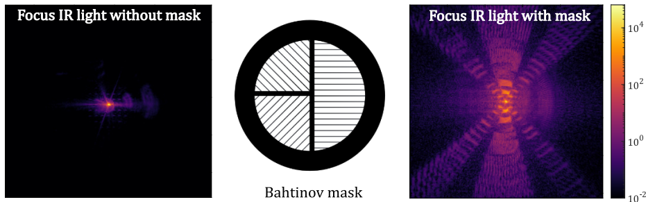
Figure 4.23: Without introducing any attenuation (or reduced repetition rate) of either the IR beam or EUV beam, capturing non-overexposed images of the beam near the focus becomes rather tricky. At a lower flux, non-overexposed images can be made without much detail due to the rather large pixels and a small probe when performing a through-focus scan. Placing a binary transmission Bahtinov mask, consisting of three sections with two diagonal gratings and one horizontal grating, as close as possible to the ellipsoidal mirror results in additional diffraction orders in the focal plane. The 0 th still closely represents the probe without a mask, but the energy is more dispersed across the camera, relieving the exposure problem. The main benefit of the mask is the ability to find the focal plane, as shown in Fig. 4.24. Note that the image on the right is on a log scale.
