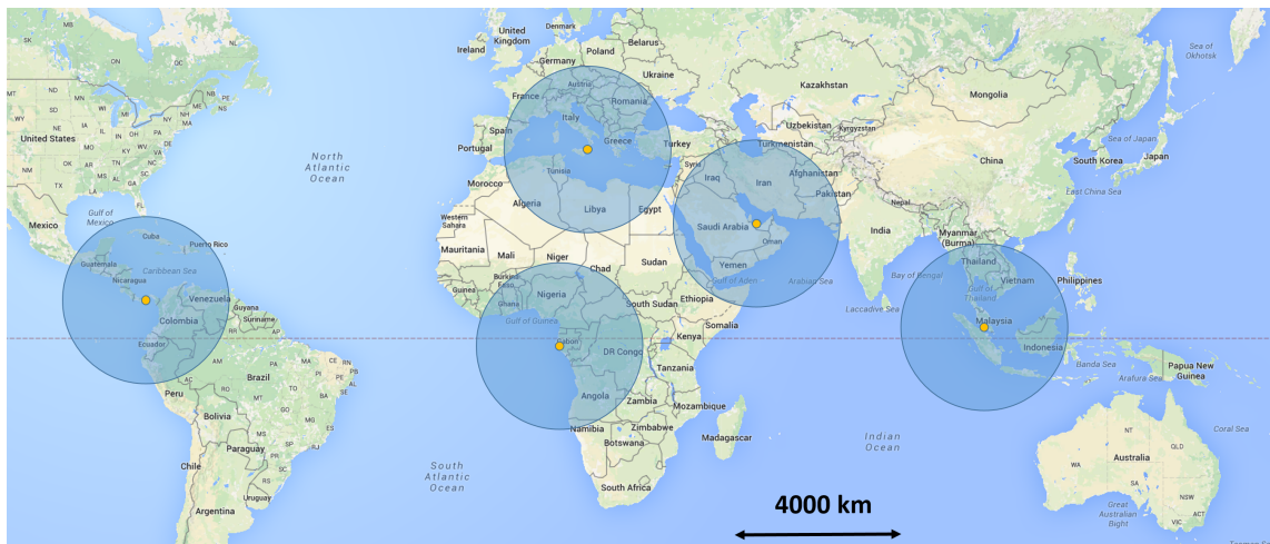
Figure 11.1: Ship range ( 2160 \text{ km} ) in 72 hours assuming an average velocity of 30 \text{ km/hr} .
