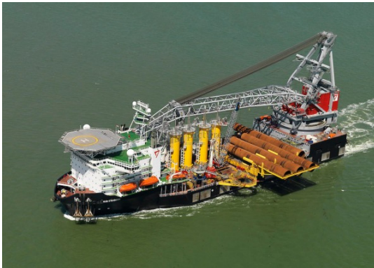
(a) Monopile transport on HLV
