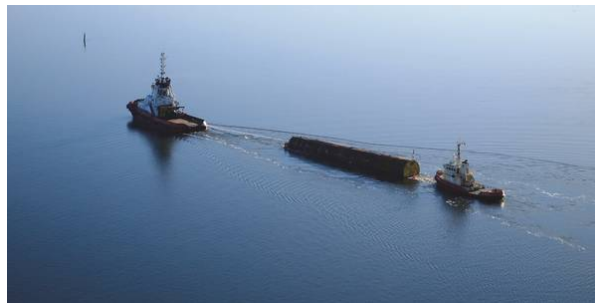
Figure 2.6: Floating delivery of monopiles using monopile end caps [15]
