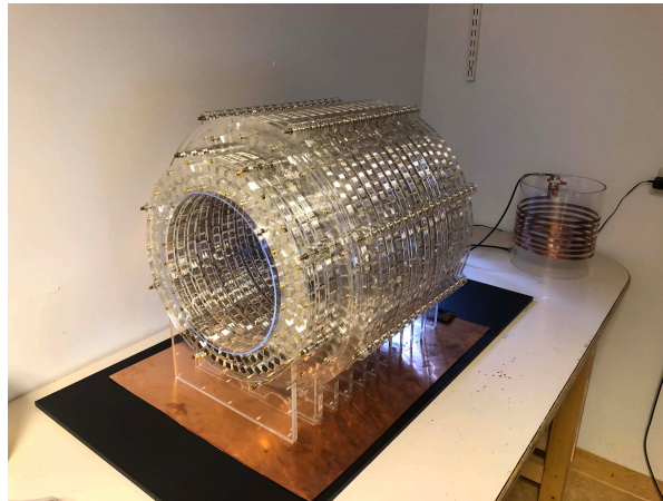
Figure 1.4: The low-field (50mT) scanner developed by O'Reilly et al. [10].
