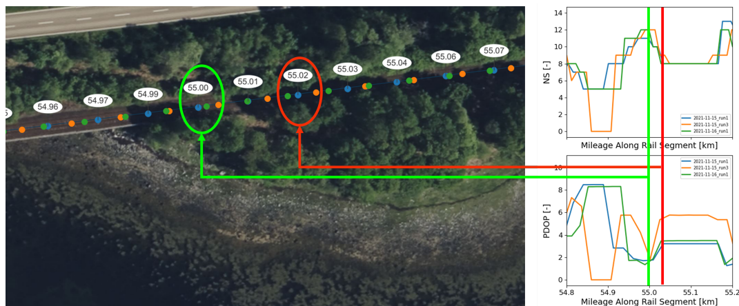
Figure 4.5: Quality metrics with corresponding location on the map, RTSS moving from 'open area' into 'vegetated area'. Train direction is from left to right.
