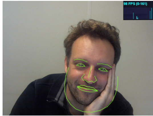
Figure 1. Face fitting model used by Clmtrackr; also shows a common fitting error due to hand positioning
